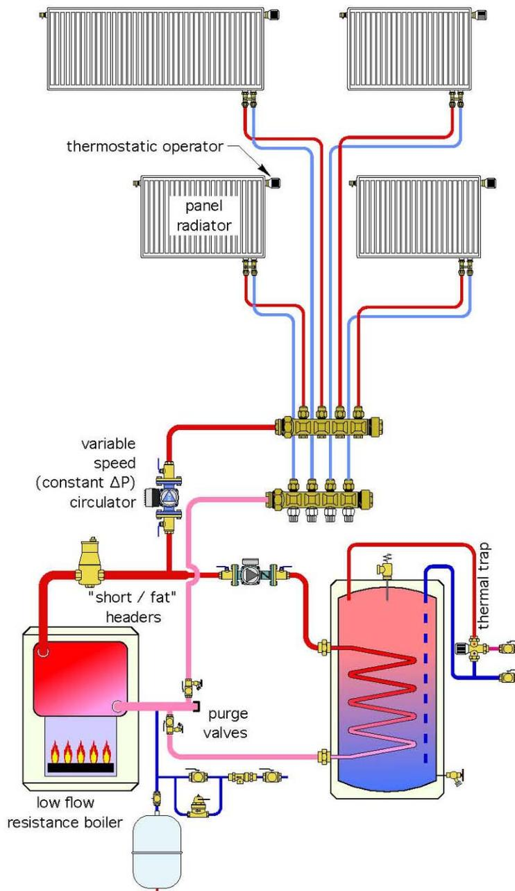
Another change is the use of a pressured regulated constant  $\Delta P$  circulator within the subsystem serving the panel radiators. This eliminates the need of a differential-pressure bypass valve and significantly reduces operating cost compared to a fixed-speed circulator.
