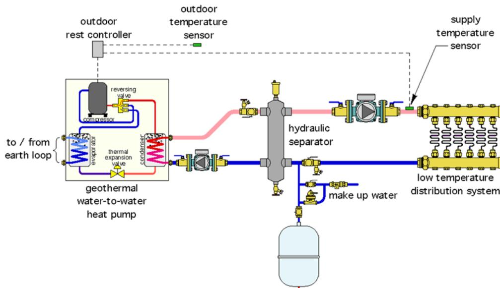
2. It makes no sense to operate the geothermal heat pump above the temperature necessary to meet the current heating load. Operating the heat pump at 125° F and mixing down the water temperature to the floor circuits just reduces the COP and heating capacity of the heat pump. This scenario also "wastes" the potential of outdoor reset control.
