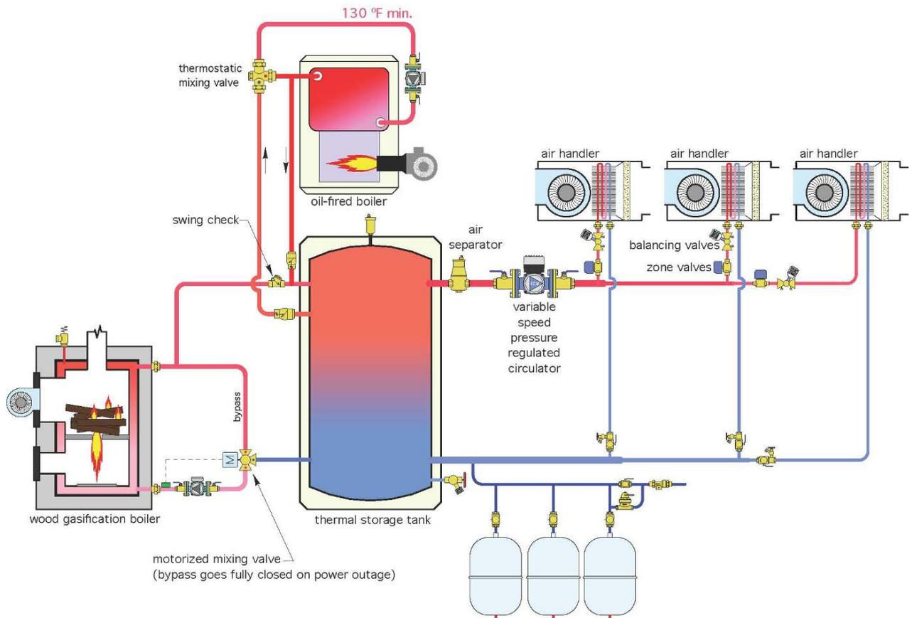
The system now includes thermal storage, the size of which needs to be calculated based on the capacity of the boiler and the allowable temperature change in the tank. A typical residential-scale wood-gasification boiler will usually require 300 to 500 gal. of storage.
