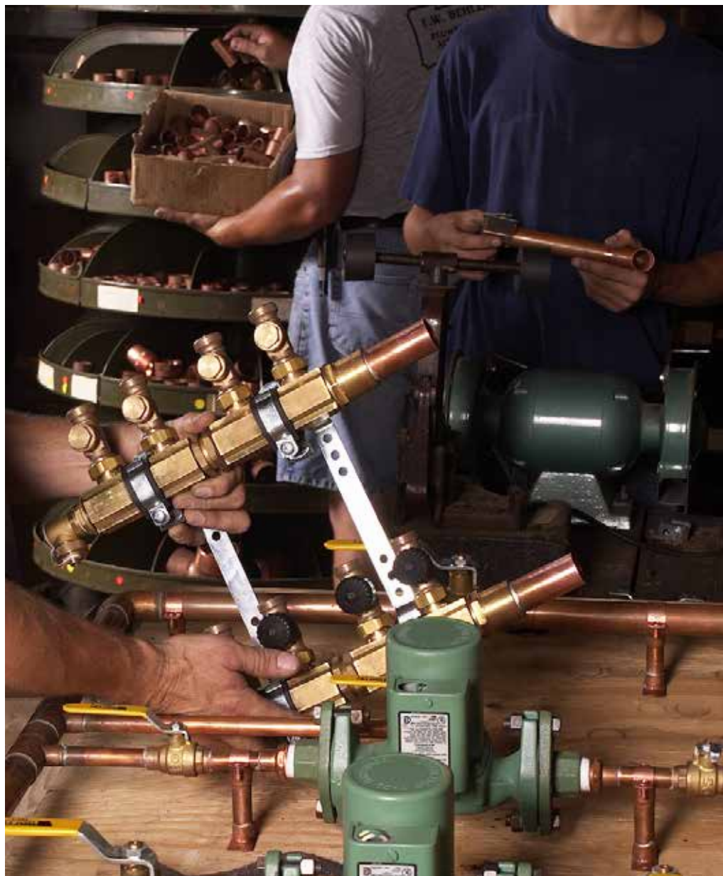
Time saved by constructing shop-built manifolds with pre-wired controls.
