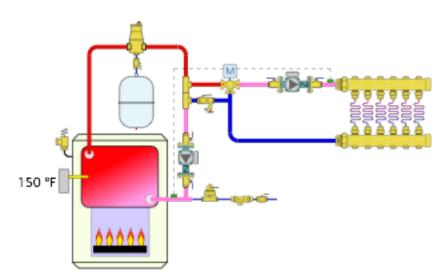
This system uses a motorized 3-way mixing valve to control supply water temperature to the floor heating circuits. The controller operating this valve monitors boiler inlet temperature and reduces the flow of hot water into the mixing valve whenever necessary to quickly establish and maintain a boiler inlet temperature of at least 130°.
