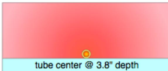
There's a 26 percent drop in heat output for tubing installed at the bottom, rather than the mid-height of the slab. If the slab needs to release heat at a rate of 15 Btu/hr/ft<sup>2</sup>, the average circuit water temperature needs to increase about 7 °F if the tubing is left at the bottom of the slab rather than placed approximately at mid-slab thickness. If the slab
