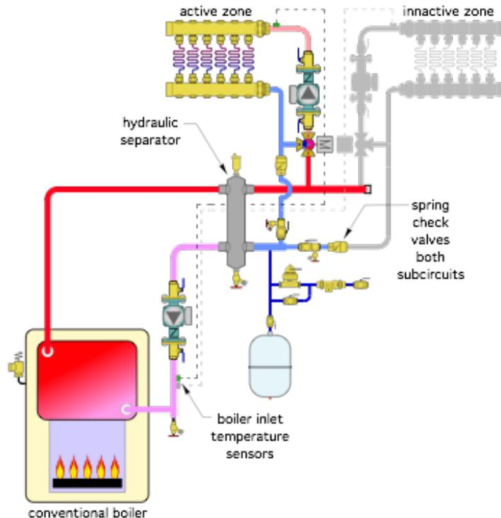
The fix drawing uses a hydraulic separator between the “boiler loop” and the two distribution sub-circuits. The upper portion of the hydraulic separator provides high performance air separation and thus eliminates the need for the air separator in the original design. The bottom of the hydraulic separator adds efficient dirt separation.
