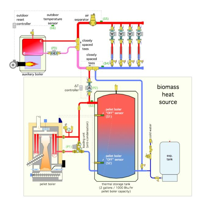
Think of the combination of the pellet boiler and thermal storage as the "biomass heat source." Whenever possible, all heat needed by the loads will come from the biomass heat source. It's injected into the distribution system at a pair of closely spaced tees. Likewise, any supplemental heat from the oil-fired boiler is injected into the distribution system at another
