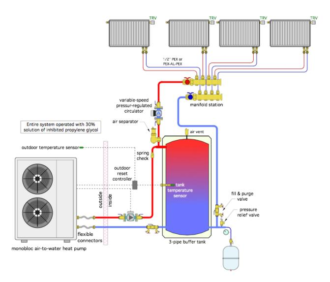
When the heat pump is enabled to operate (typically at beginning of heating season, and for the duration of that season), it monitors the temperature of the buffer tank sensor. The fixed temperature cycling range of 120° to 130°, although attainable, is relatively high for most air-to-water heat pumps. Operating at those conditions will lower the heat pump's COP. This has been changed in two ways.
