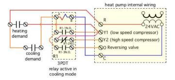
**HEATING MODE:** When the heating demand contact closes, 24 VAC from the (R) terminal passes to the (Y1) terminal. From (Y1) 24 VAC also passes through the normal closed relay contact (R1-2 N.C.) to energize the (Y2) terminal. The heat pump is now running in full capacity heating mode.
