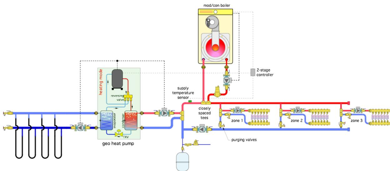
Each manifold station is also supplied from a pair of closely spaced tees installed in parallel “crossovers” of the primary loop. This keeps the supply water temperature to each manifold station approximately equal. The system has a seven identical 1/25 HP circulators.
