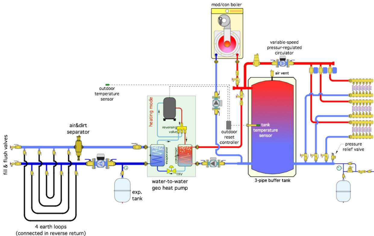
Both heat sources can operate individually or in parallel supplying heat to a buffer tank. The mass of the buffer tank stabilized the system against short cycling.
