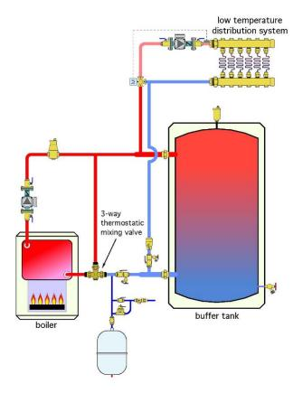
A high flow capacity, three-way thermostatic mixing valve is used to protect the boiler from low entering water temperatures.
