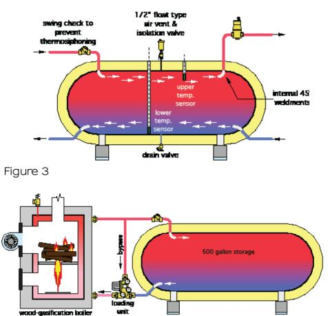
remedied by welding additional threaded pipe bosses to the tank shell where needed. This welding can be done to ASME Section VIII standards when necessary to meet local codes. I like to specify connections as shown in Figure 2.
